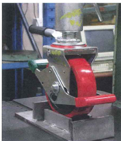
Figure 1: The loading of the castor in the test machine
