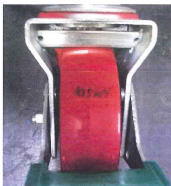
Figure 2: The depressions on the wheel after the application of the load. The load applied for the impression shown is marked on the photograph: 10.5kN for 1.5 times the rated load and 21.0kN for 3 times the rated load
