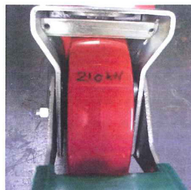
Figure 2: The depressions on the wheel after the application of the load. The load applied for the impression shown is marked on the photograph: 10.5kN for 1.5 times the rated load and 21.0kN for 3 times the rated load
